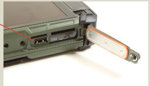
With door open - USB 2.0 Host x 1, SD (SDHC) card slot x 1, - SIM card slot x 1
